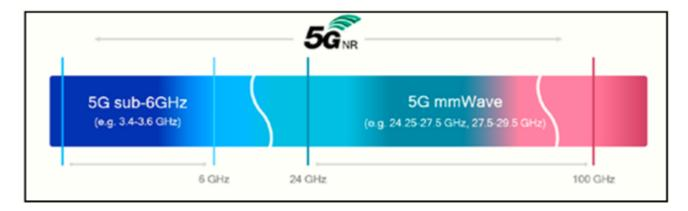
On Figure 1 shows extended spectrum for 5G NR.
